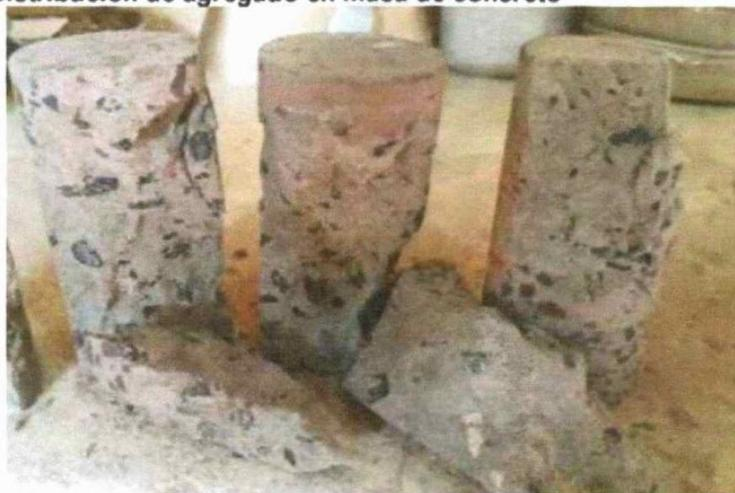
**Figura 19. Muestra ensayada a compresión simple.**
